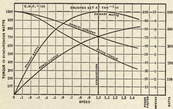
Fig. 103.—Characteristics of Ideal Repulsion Motor.
