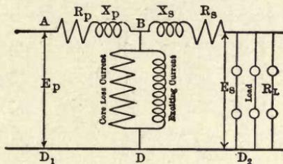
FIG. 47.—Equivalent Electric Circuits of an Ideal Transformer.
