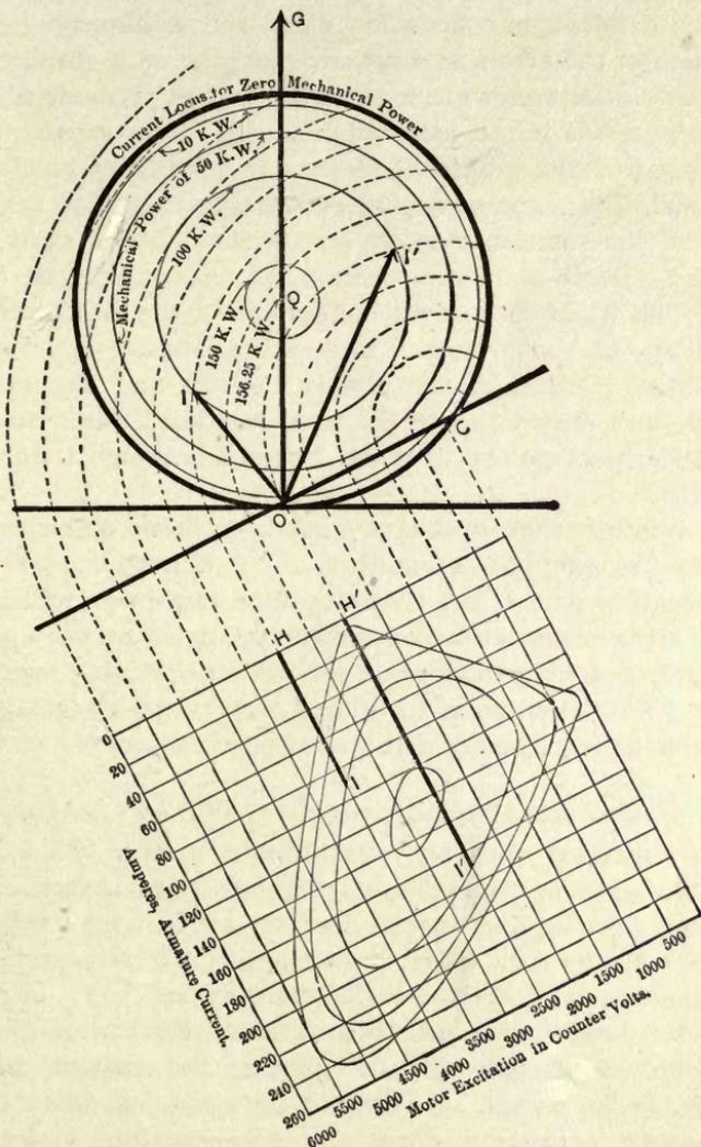
FIG. 94.—Circular current loci; O-curves and V-curves.
