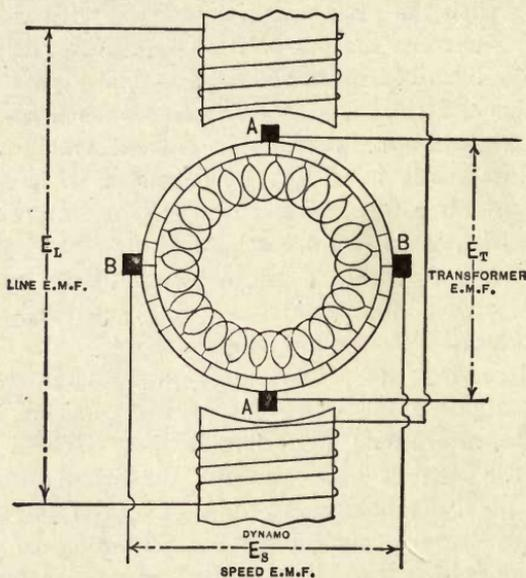
FIG. 105.—Electromotive Forces Produced in an Alternating Field.
