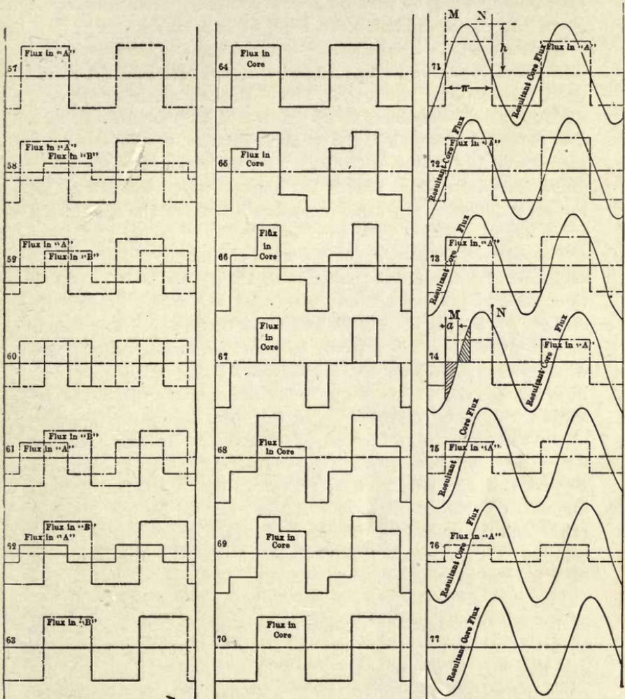
FIGS. 57-63.—Flux Demanded by each Phase; Secondary open.
