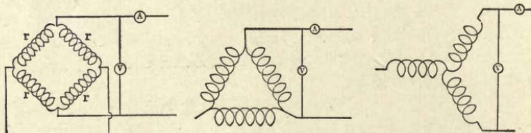
FIGS. 13, 14 and 15.—Determination of Equivalent Single-phase Resistance.
