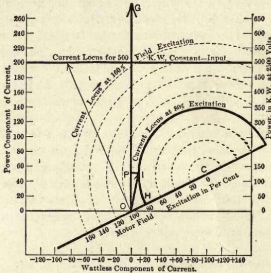
FIG. 92.—Circular current loci for various motor excitations.
