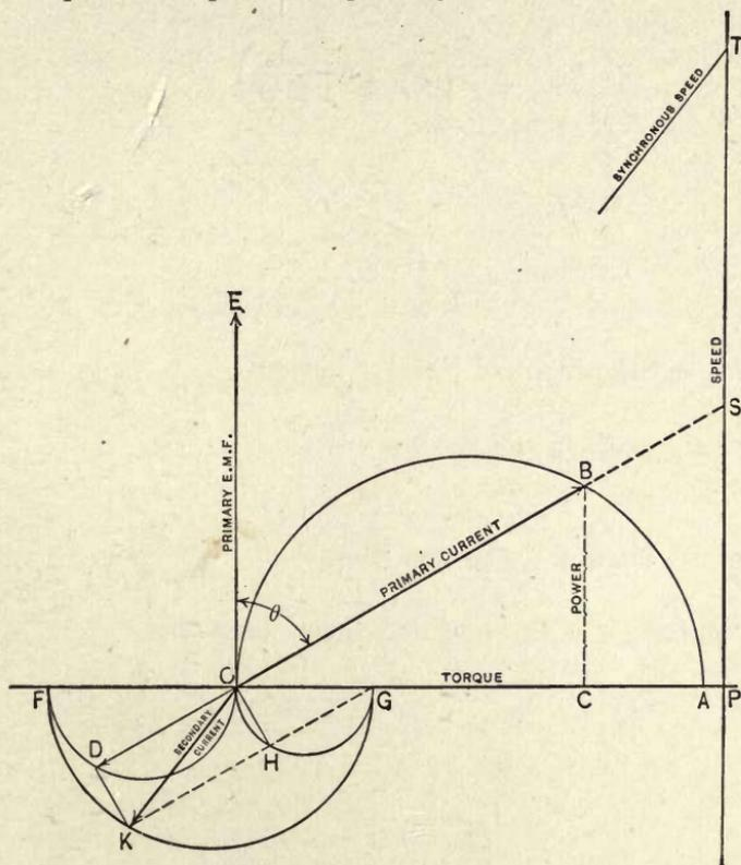
FIG. 107.—Vector Diagram of Ideal Repulsion Motor.
