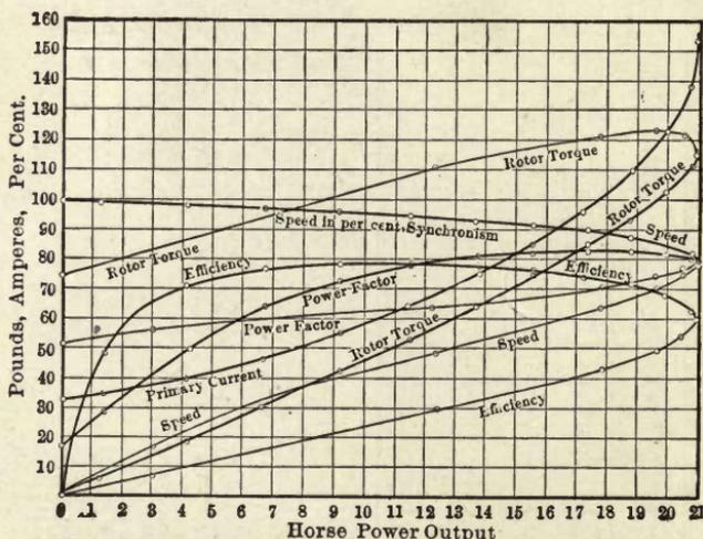
FIGS. 36 and 37.—Performance of Two-phase Induction Motor.
