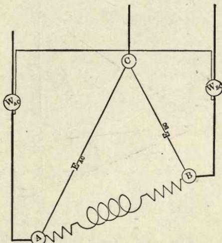
FIG. 5.—Measuring power in coil  $A B$ .
