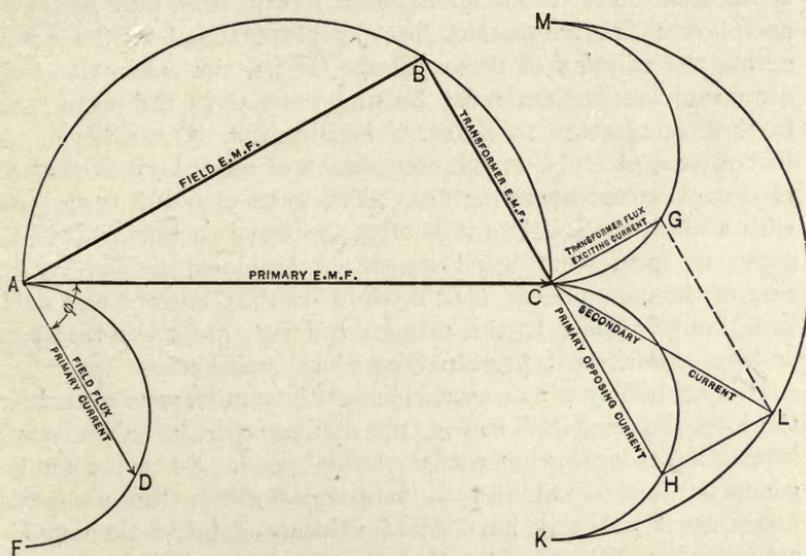
FIG. 102.—Vector Diagram of Ideal Repulsion Motor.
