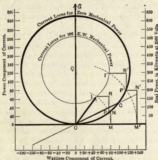
FIG. 93.—Circular current loci for various mechanical loads.
