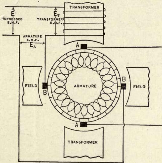
FIG. 109.—Two-pole Model of Compensated Repulsion Motor.
