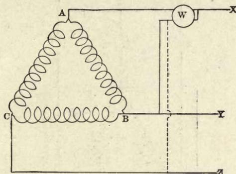
FIG. 7.—Measuring three-phase power with one wattmeter.
