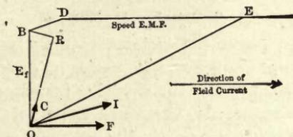
FIG. 132.—E.m.f.-current Locus of High Power-Factor Non-sparking Motor.
