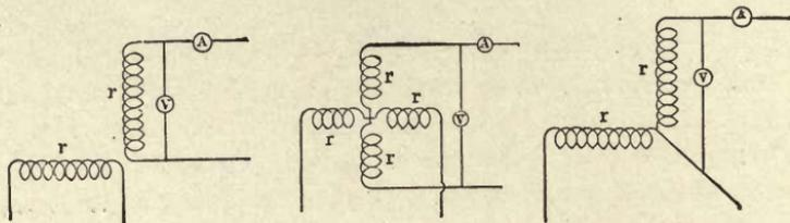
FIGS. 10, 11 and 12.—Determination of Equivalent Single-phase Resistance.
