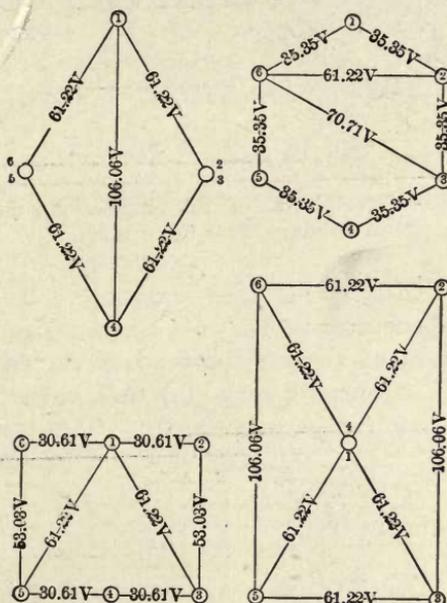
FIGS. 90 A, B, C, and D.—Symmetrical Voltage Diagrams.
