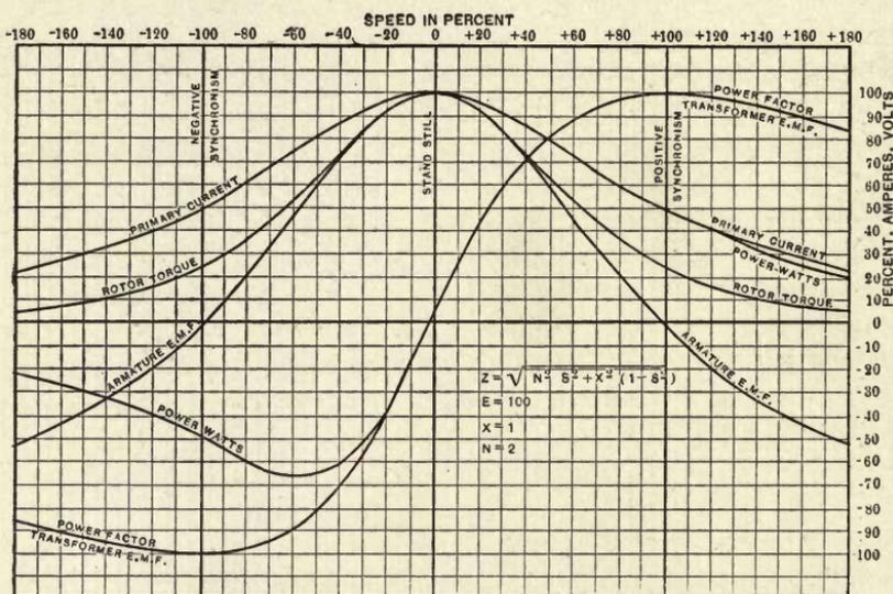
FIG. 111.—Characteristics of Ideal Compensated Repulsion Motor.
