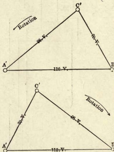
FIG. 32.—Diagram of Three-phase e.m.f.'s.
