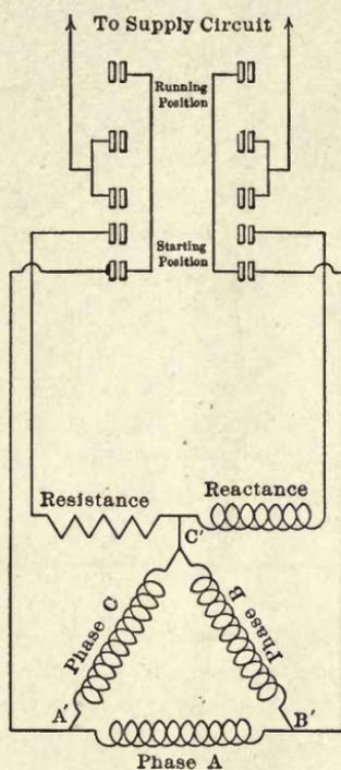
FIG. 30.—Circuits of (Three-phase) Single-phase Motor.
