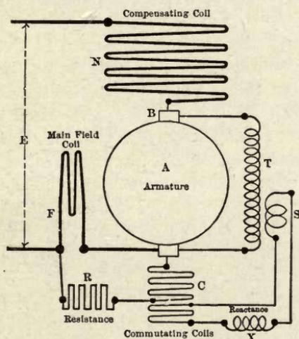
FIG. 133.—Automatic Non-sparking, High Power-Factor Motor.
