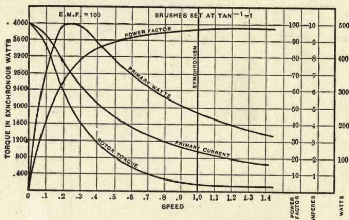
FIG. 104.—Characteristics of Ideal Repulsion Motor.
