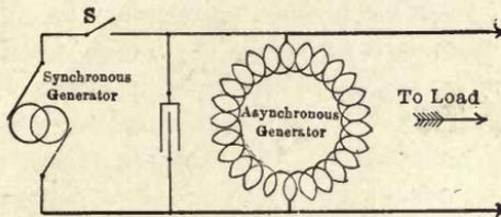
FIG. 41.—Asynchronous Generator; Condenser Excitation.
