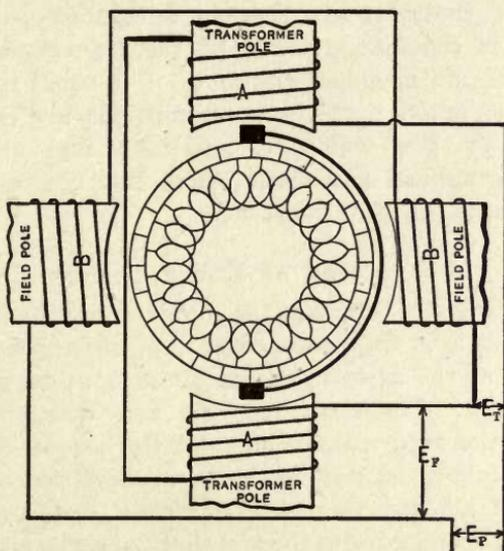
FIG. 101.—Circuits of Ideal Repulsion Motor.
