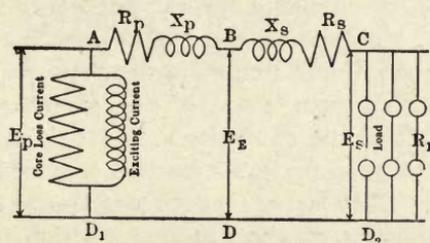
FIG. 136.—Simplified Circuits of Induction Motor.
