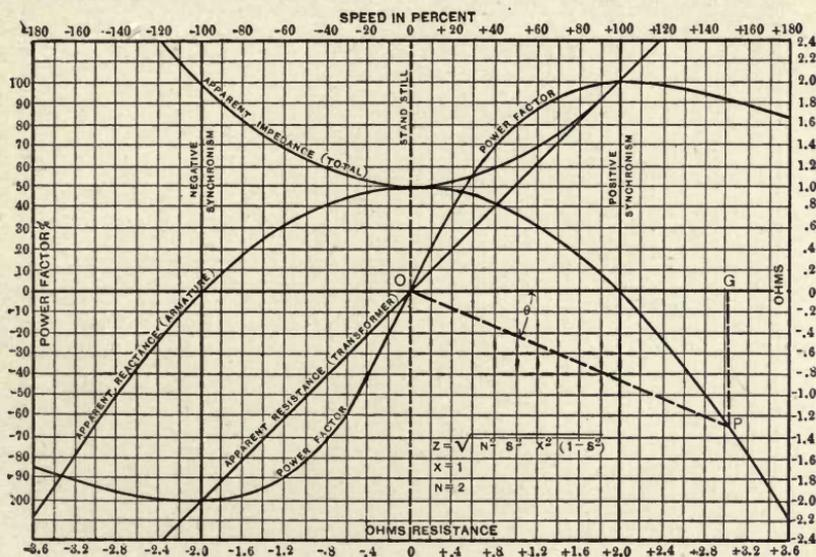
FIG. 110.--Characteristics of Ideal Compensated Repulsion Motor.
