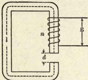
FIG. 78A.—Simple Magnetic Circuit.
