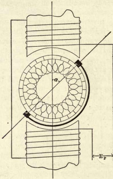
FIG. 100.—Circuits of Repulsion Motor.
