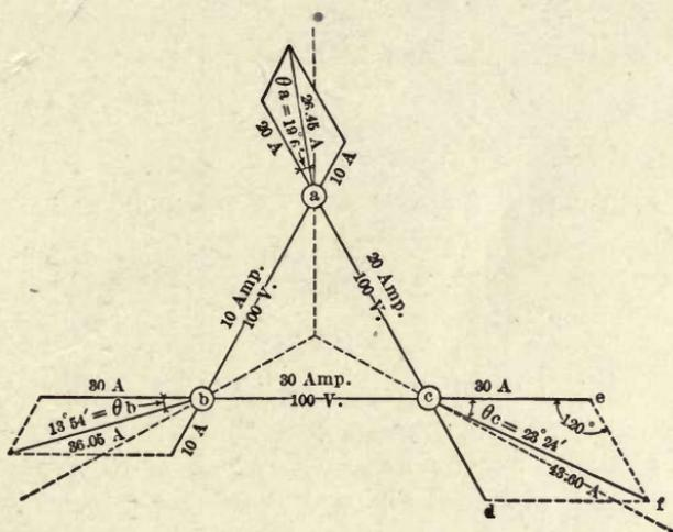
FIG. 9.—Vector Diagram of Currents and Electromotive Forces.
