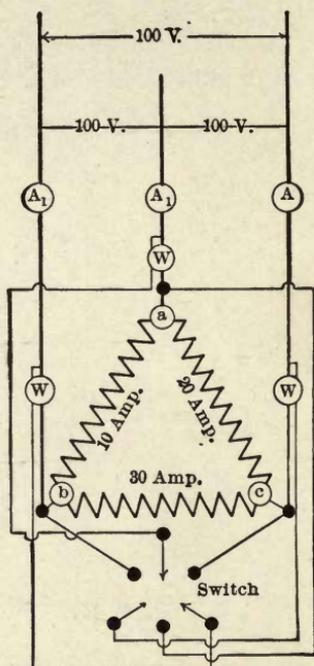
FIG. 8.—Testing Circuits.
