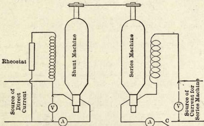
FIG. 99.—Determination of Torque.
