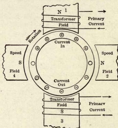
FIG. 79.—Production of "Speed-field" Current.
