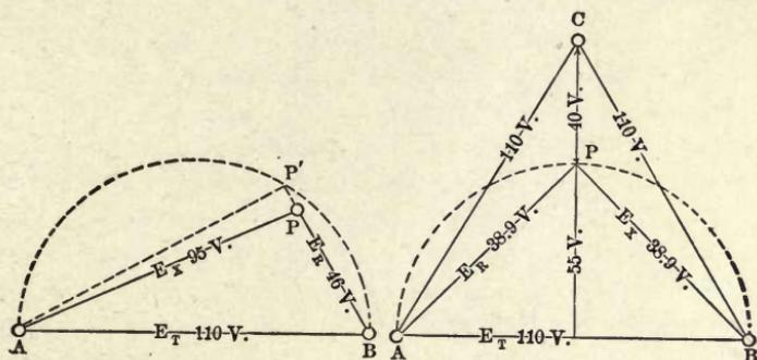
FIGS. 33 and 34.—Vector Diagram of Electromotive Forces.
