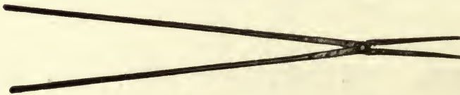
FIG. 12.—Crucible tongs for use in gasoline melting-furnace.
